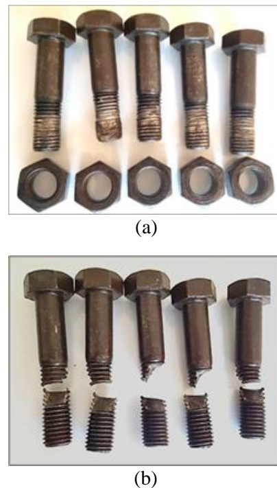
Fig. 1. Failure patterns: (a) Tensile test by nut, (b) Tensile test by ISO 898-1 device
